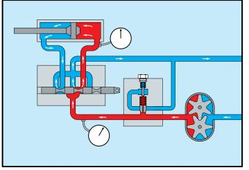
Here is why. Suppose that in this conventional system the pump is producing 20 GPM and the valve spool is moved to direct part of pump flow to the cylinder and part to tank. The flow of oil past the control spool causes a certain pressure drop. That pressure drop can be felt by the operator in the effort required to move the valve spool control lever.
