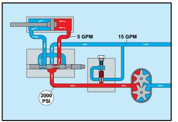
That means, in this system, 17.5 horsepower times 42.4 BTU's or 742 BTU's of heat per minute must be absorbed by the hydraulic system and, eventually, dissipated through an oil cooler.
