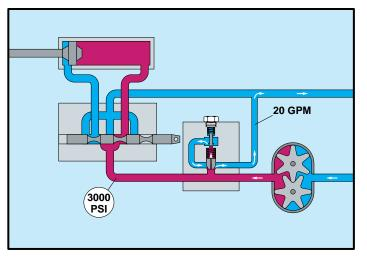
Here is the conventional system again, but this time it is shown in the relief position. The piston in the cylinder has reached the end of its travel and all pump flow is passing through the system relief valve that is set at 3000 PSI. 3000 PSI times 20 GPM divided by 1714 shows that 35 horsepower is wasted in by-passing oil through the system relief valve.
