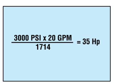
35 Hp x 42.4 BTU = 1484 per min. or 89,040 BTU per hour 35 horsepower times 42.4 BTU's per minute equals 1484 BTU's of heat that is generated unnecessarily every minute or 89,040 BTU's per hour.
