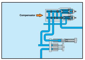
This is the compensator which monitors the system and controls the performance of the pump.
