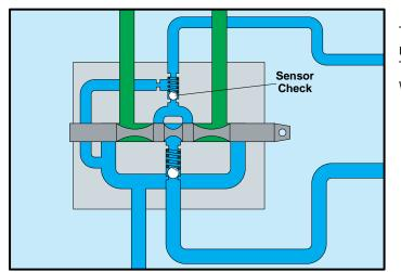
The valve also has a sensor check. When the system has more than one spool, there is a sensor check for each spool. The check allows the compensator to adjust itself to the circuit which calls for the highest pressure.
