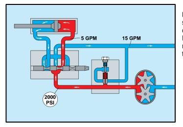
Here is a typical open center, fixed displacement hydraulic system. The pump can produce 20 GPM. Suppose the operator wants to meter oil to the cylinder that requires 2000 PSI to move the load. If only 5 of the 20 GPM are required to move the cylinder at the desired rate, 15 GPM are returned to tank. However, the full 20 GPM is pressurized to 2000 PSI.
