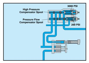
It contains a high pressure compensator spool that works against a 3000 PSI spring; and a pressure-flow compensator spool that works against a 200 PSI spring. The compensator is mounted directly on the pump.
