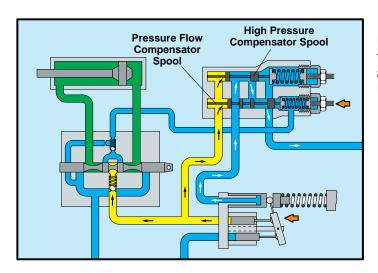
Pump flow also enters the pump compensator. It acts against the left end of the pressure-flow compensator spool and against the left end of the high pressure compensator spool. Remember that all this takes place in a split second.
