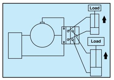
In the conventional system, the actuator with the least load will move first, then the other.
