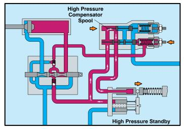
Remains in high pressure standby until the load is overcome or the valve spool is returned to neutral. The Eaton pump will remain in high pressure standby until (1) The load is overcome or (2) The valve spool is returned to neutral. It will produce only enough flow to make up for internal leakage.
