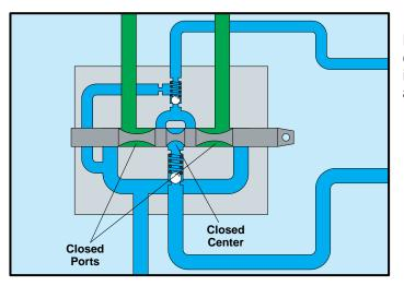
Notice that the directional control valve is the closed center, closed port type. This means that when the spool in the valve is centered, pump flow is blocked at the entrance to the valve and both ports which lead to the cylinder are also blocked
