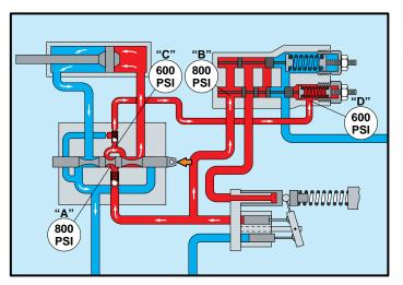
If we install those four gauges again we see that, even though the resistance created by the spool passage is less and the pump is producing move flow, there is still exactly 200 PSI difference in pressure between the two sets of gauges. The pressure-flow compensator spool will always strive to maintain this 200 PSI difference while the spool in the directional control valve is moved to direct oil to an actuator.
