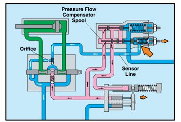
Notice that the spring chamber at the right of the pressureflow compensator spool is drained of oil. This oil flows from the spring chamber to the directional control valve.
