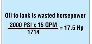
17.5 horsepower is wasted in returning oil to the tank.
