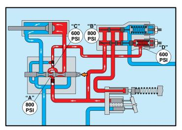
In the Eaton system it doesn't make any difference how far the control valve spool is moved. The compensator will always adjust pump flow so that there is exactly a 200 PSI pressure drop across the spool.
