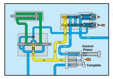
Because there is no oil pressure acting against the control piston, it forces the camplate to move to its maximum angle. In this position, the pump is ready to produce maximum flow.
