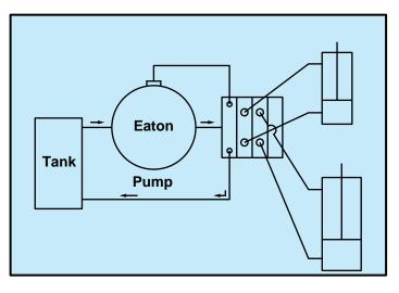
In the Eaton system the pump adjusts itself to the flow requirements of each circuit.
